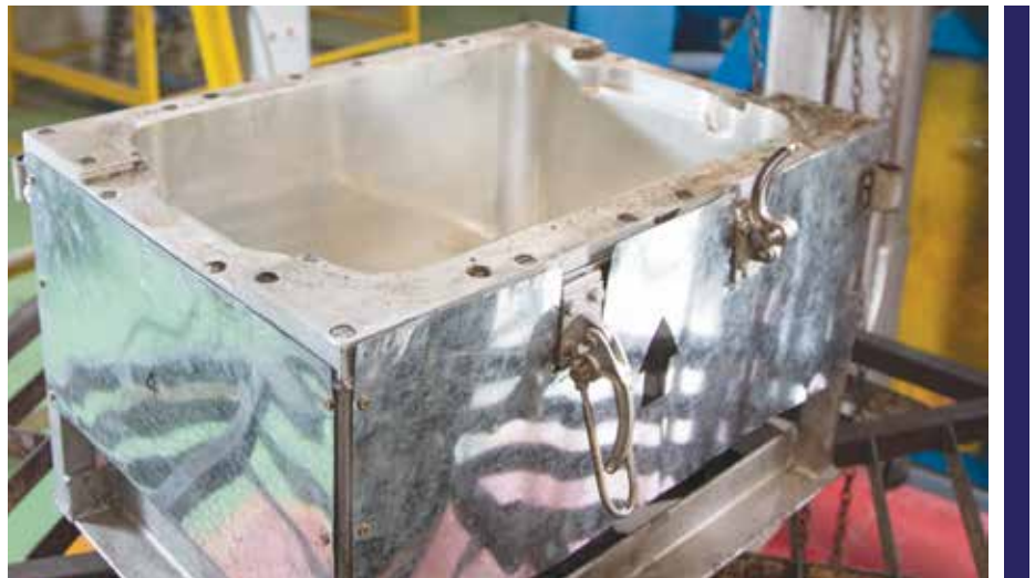
■ Heat Shielding by Metal Sheet on Exterior Surface of The Mold
